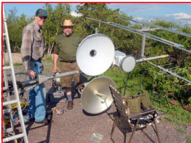
**WA3RLT and WA3GFZ attaching the 10GHz feed**
